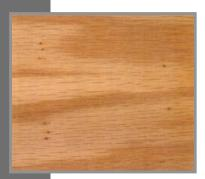
■ PIN KNOTS: Sound knots 6.4 mm (1/4 inch) or less in diameter containing dark centers.
