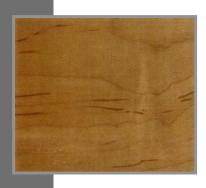
WORM TRACKS: Marks caused by various types of wood attacking larvae. Often appear as sound discolorations running with or across the grain in straight to wavy streaks.
