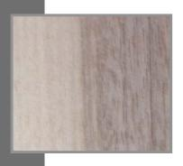
■ **SAPWOOD:** The living wood of lighter color occurring in the outer portion of a tree, sometimes referred to as sap.
