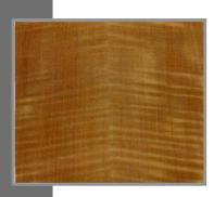
■ CROSS BAR (FIGURE): Irregularity of grain resembling a dip in the grain running at right angles, or nearly so, to the length of the veneer.
