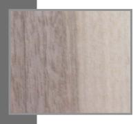
■ **HEARTWOOD:** The non-active or dormant center of a tree, generally distinguishable from the outer portion (sapwood) by its darker color, sometime referred to as heart.
