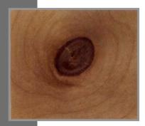
■ KNOTS: Cross section of tree branch or limb with grain usually running at right angles to that of the piece of wood in which it occurs.
